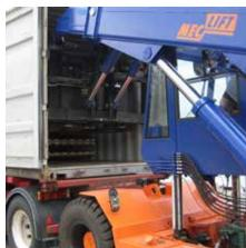
"We use two Meclift ML1812R machines for loading and unloading steel coils into and out of containers in our port. These machines are very unique in design. Thanks to their low height and good reaching ability we are able to use them in other jobs as well. Sometimes we wonder how some of these jobs could be done without the Meclift trucks."
