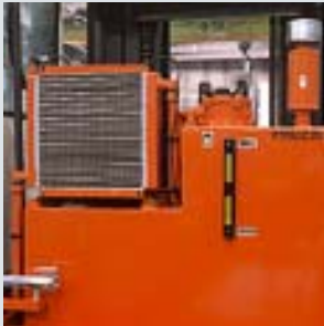
Hydraulic oil cooling system
