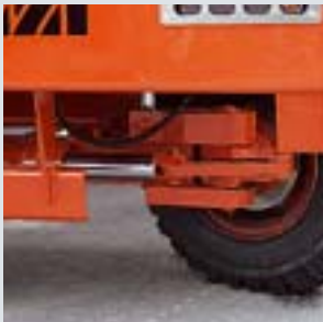
Dry disc brakes on steering wheels
