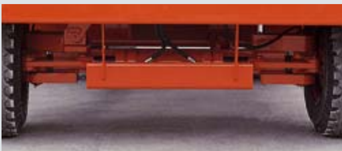
Single "double acting" steer cylinder
