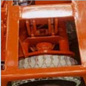
Wheel mounted drive hydromotors
