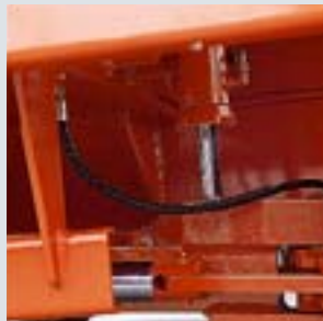
Tilt cylinders on operator's side
