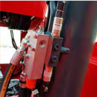
Detection of load weight through 4 pressure transducers: 2 placed on lifting cylinders and 2 on compensation cylinder.
