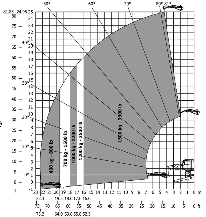
Rotation on lowered stabilisers with 365 kg platform
