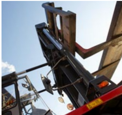
Full visual contact with the load and attachment, is provided by the Spirit Delta cabin and the open design of the mast and carriage.
