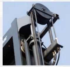
The DCF80-100 has considerably fewer hoses over the mast compared to conventional machines (2 hydraulic hoses and 1 electrical cable). This provides greatly improved functional reliability.
