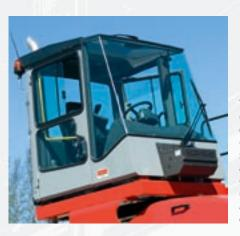
The Spirit Delta cab has an electronically controlled heating system (ECH) as standard. A climate system (ECC) is also available as an option.
