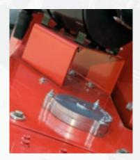
The fine filter in the hydraulic system maintains the oil's performance longer and extends the life span.
