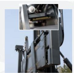
The levelling of the twistlock attachment is now enabled in the main attachment rather than at the twistlock. The construction is now far simpler and offers increased reliability.
