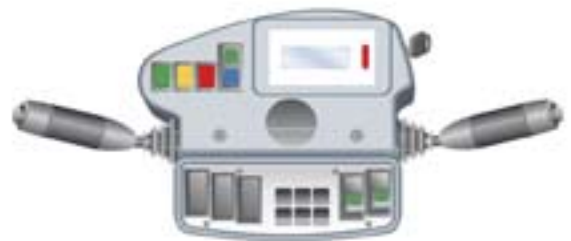
Levers for hydraulic functions: Lifting, tilt, side shift, 20-40 feet extension, twistlocks/flaps.
