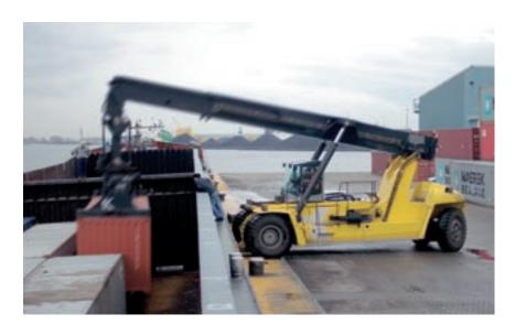
The boom's lifting and extension cylinders are fitted with double gaskets. Moreover, the machine is fitted with extremely reliable, well-sealed ORFS (O-Ring Face Seal) couplings in all the hydraulic hoses as standard.
