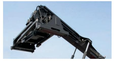
The boom requires a minimum of mainenance due to lubriaction free sliding plates.
