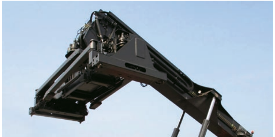
The boom requires a minimum of maintenance due to lubrication free sliding plates.
