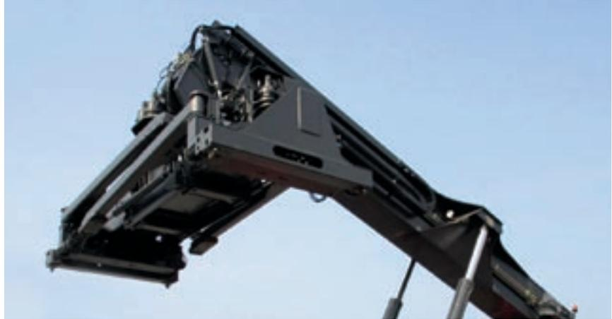
The boom requires a minimum of maintenance due to lubrication free sliding plates.
