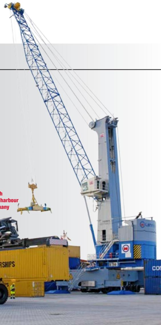
Terex reach stackers interact with a Terex Gottwald Model 5 mobile harbour crane at the Port of Lübeck, Germany
