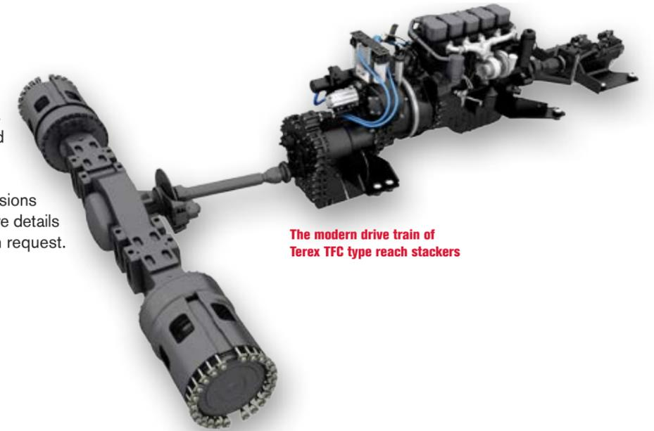
The modern drive train of Terex TFC type reach stackers
