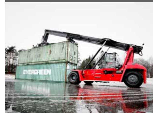
Precise lifting of long container end-on - 40 ft
