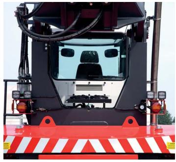
he manually sliding cab leaves complete access to the engine and transmission bay and routine maintenance tasks are made easier by conveniently repositioned fluid level refill cum check points and filters. The roomy Electric System compartment contains and protects the already all-wether proof IP 67 main electric box and system components.
