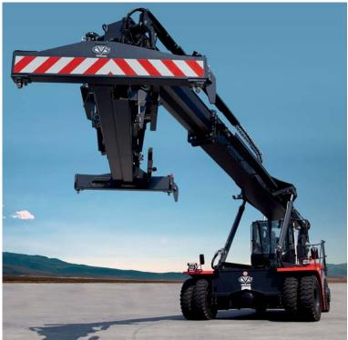
he all high tensile strength light and super strong spreader enables RSE to grant full second and third row and to handle "end on" 40' even 45' containers in full safety and guarded by a computer managed boom-spreader anti-collision device. The spreader has a generously sized rotation gear, moved by two large gear reducers and motors and it is stepless controlled by the truck on board in its rotation and side-shift motions.
