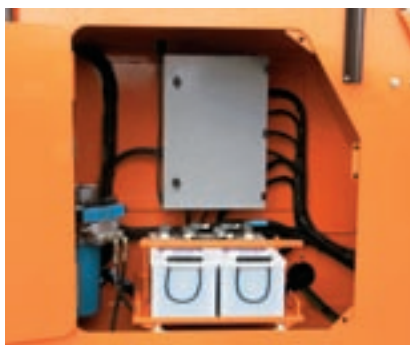
Service hatch on right hand side. The batteries can be rolled out.
