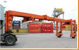
Compact design enables operating through terminal door openings.
