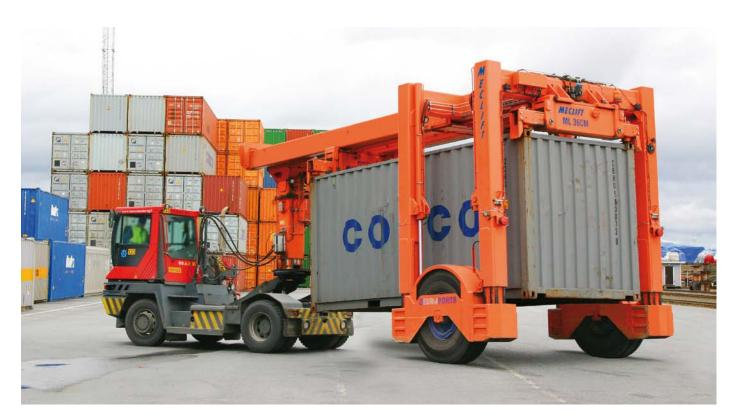
The efficiency of the Meclift Container Mover ML36CM is proven daily at the Rauma Stevedoring port. The costs in horizontal container moving are only a half of similar operation by means of a reach stacker. In addition, longer transportations can be done with ML36CM only, without any other machinery. Improved work safety and ergonomics enhance smooth operation. Certain technical requirements taken into consideration, the machine can be attached to any terminal tractor.
