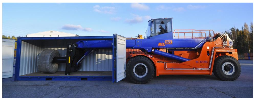
With high reaching capability, **Meclift<sup>TM</sup> ML4212RC can reach to the end of a standard 20" container and still lift 10 tons**, making all logistical maneuvers significantly easier and safer.
