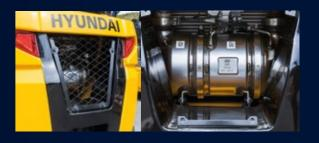
For greater convenience, the counterweight opening has been made as large as possible. This **eliminates the need to remove the counterweight** for inspection or exchange of the after-treatment device.
