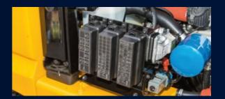
All fuses and relays are centralized in three boxes with **enhanced waterproof and dustproof protection IP65**. The boxes themselves are located behind the side cover panel for **quick access**.
