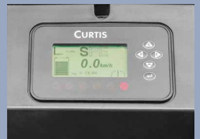
Standard LCD display informs the driver about all necessary informations
