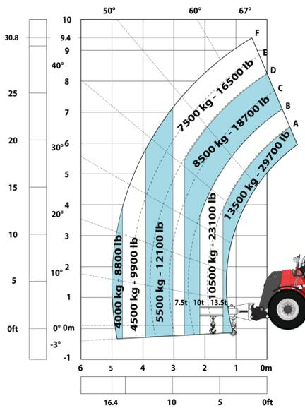
Machine on tyres with tyre handler TH 51 (Metric)
