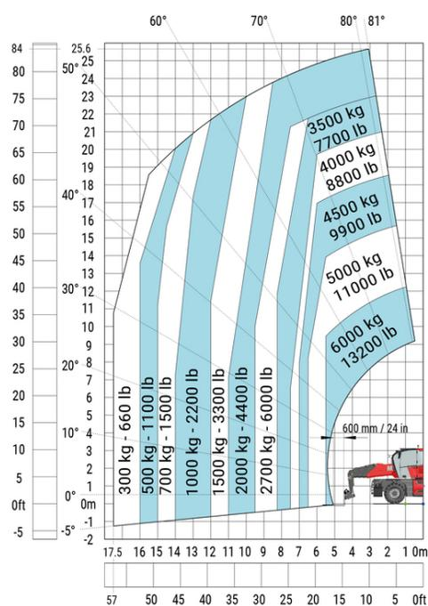
Machine on lowered stabilisers with 600 kg jib (Metric)
