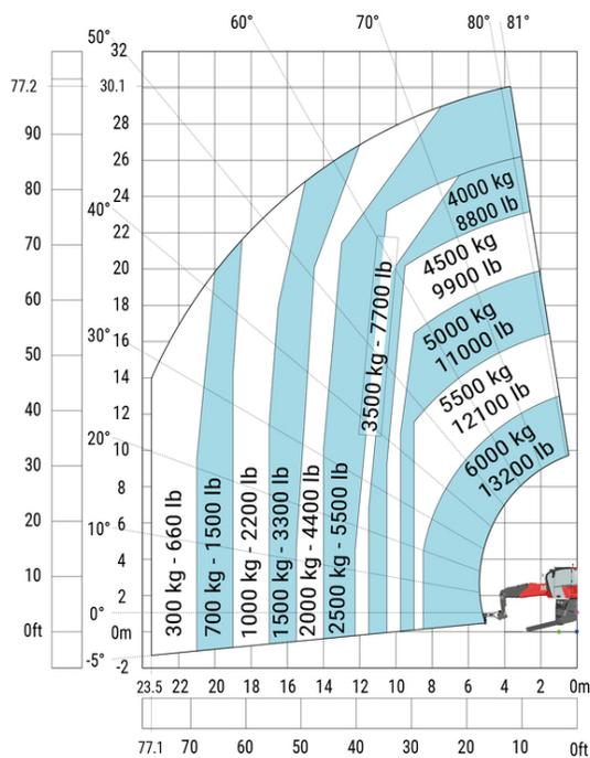
Machine on lowered stabilisers with 2000 kg jib with winch (Metric)
