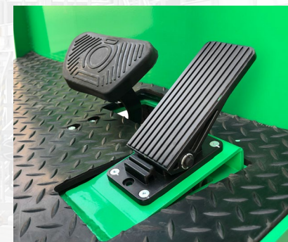
Large Brake Pedal with Integrated Parking Brake Design
