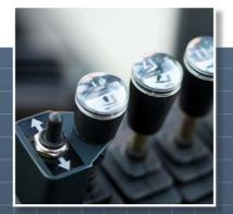
ever with forward/reverse control Allows you to change direction by simply switching the lever. Perfect when operating the machine in narrow spaces, with frequent changes of direction
