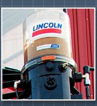
Central greasing Automatic greasing o the machine's greasing points. Prolonas the life time of the components
