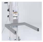
STANDARD FORKS accommodate various loads for widen from 28 to 76 cm (11 to versatile lifting. Get an additional 51 cm (20 in) of lift by turning over and re-pinning the forks.
