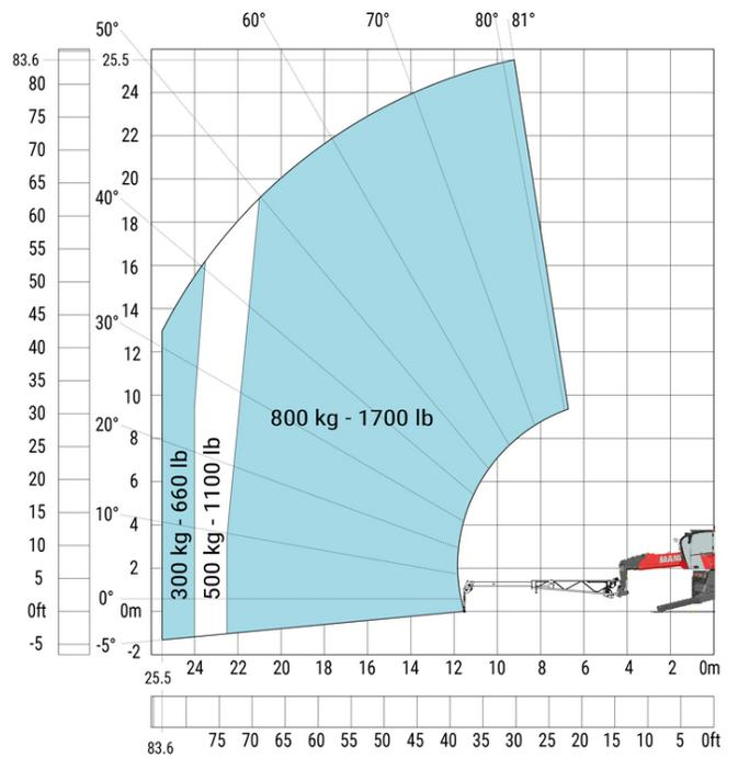
Machine on lowered stabilisers with hook 6000 kg (Metric)      Machine on lowered stabilisers with winch 6000 kg (Metric)
