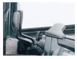
Kick-down switch is conveniently located on the boom lever. A simple motion of the thumb actuates this valuable productivity feature.
